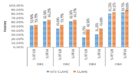
Figure 11. Accuracy of classification using k -means as descriptor clustering (10 visual word, exponential distribution of CLAHE, clip limit 0.001).
