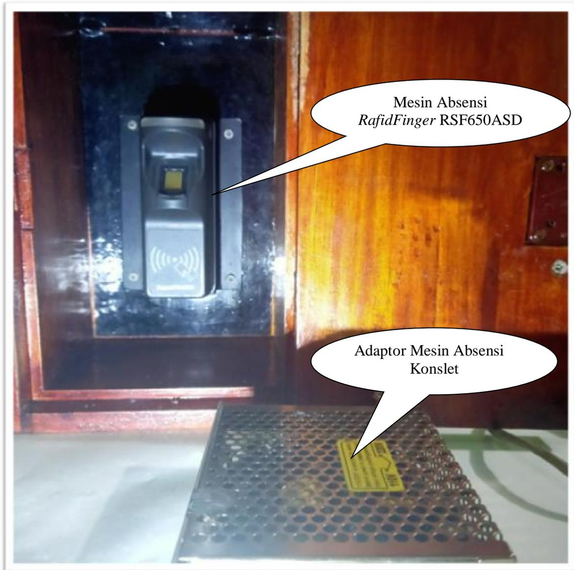
Gambar 31: Trouble Mesin Absensi fingerprint RapidFINGER RSF650ASD konslet
