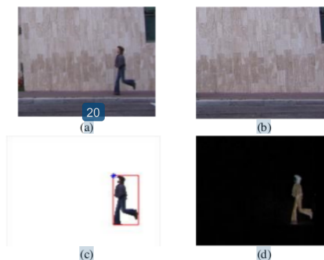
Fig. 2. Moving objects Detection using Background Subtraction (a) Current frame (b) previous frame (c) detection Object with bounding box (d) subtraction frame
