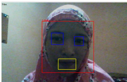
Figure 3. Face detection on dim condition In figure 3, the eyes are detected as the darkest part of the object
