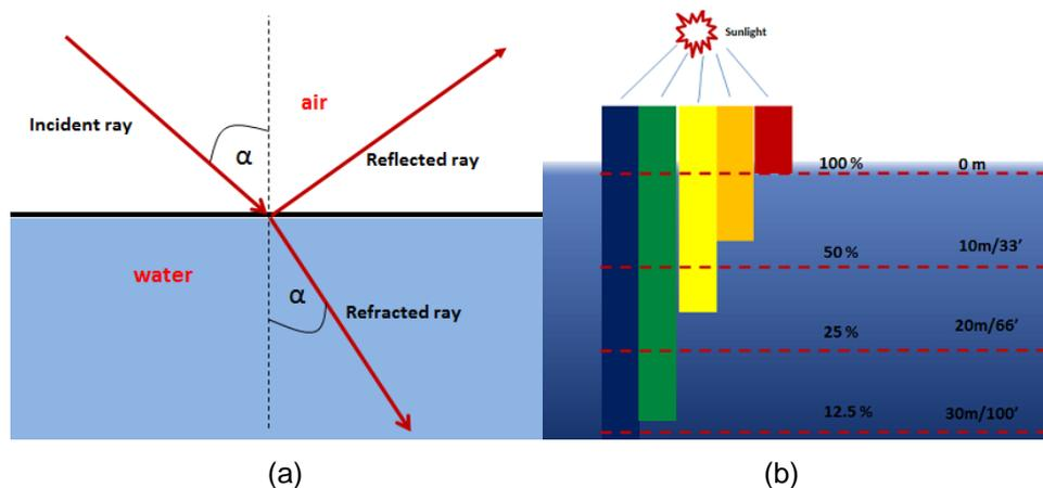
**Figure 1. (a). Water Surface Effects and (b). Absorption of Light by Water**
