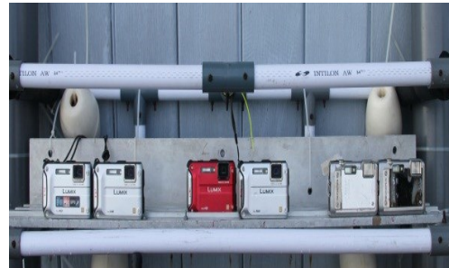
Fig. 4 Low Cost Multi-View Camera Installation
