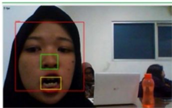
Figure 5. Face detection on bright condition In figure 3 the value is 7fps, while figure 4 and 5 each has value 3fps
