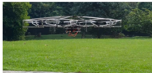
Fig. 11. First flight of heavy-lift hexacopter
