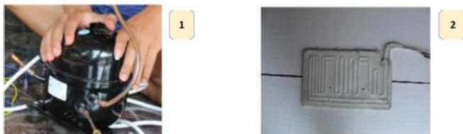
Figure 9 Compressor (1) and Evaporator (2)
