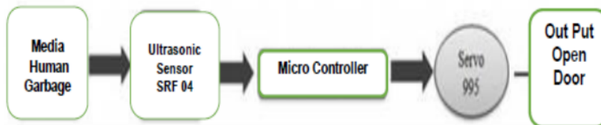
Figure 5 Automatic door working system
