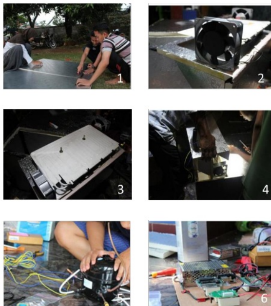
Figure 10 Cutting PIU (1), fan installation (2), installing evaporator and tool into prototype (3, 4) and installation of electrical devices on the compressor (5, 6)
