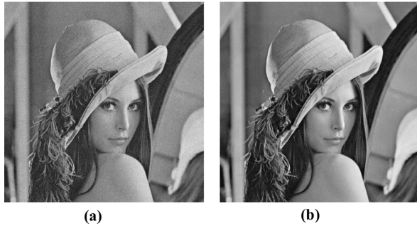
Figure 3. Noisy and De-noised Image of Lena 512×512 . (a) Noisy Image ( \sigma=10 , PSNR=28.1319dB, MSE=99.9748), (b) De-noised Image ( \alpha=0.25 , PSNR=37.1985dB, MSE=12.3945)
