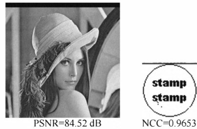
Figure 9. Watermarked image and recovered watermark after image cropping (10 rows of cropped area)
