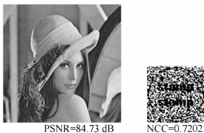
Figure 13. Watermarked image and recovered watermark after image resizing ( scale factor=2x )
