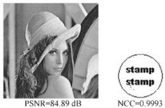
Figure 7. Watermarked image and recovered watermark after JPEG Compression ( Q=50 )
