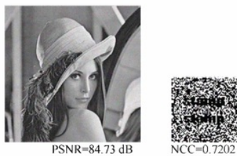
Figure 13. Watermarked image and recovered watermark after image resizing (scale factor=2x)
