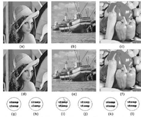
Fig. 5. Watermarked image and recovered watermark after JPEG compression ( Q=50 ); (a)-(c) watermarked image with DCT, (d)-(f) watermarked image with FWHT-DCT, (g)&(h) recovered image from (a)&(d), (i)&(j) recovered image from (b)&(e), (k)&(l) recovered image from (c)&(f).
